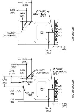
TOP VIEW - OPERATOR END ALL CONNECTIONS LOCATED UNDERSIDE OF BASE
